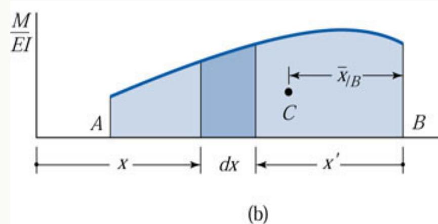
The right-hand side of Eq.(c) represents the first moment of the shaded area of the  $M/(EI)$  diagram in Fig. 6.5 (b) about point B. Denoting the distance between B and the centroid  $C$  of this area by  $\bar{x}/B$  (read /B as “relative” to B”), we can write Eq.(c) as
