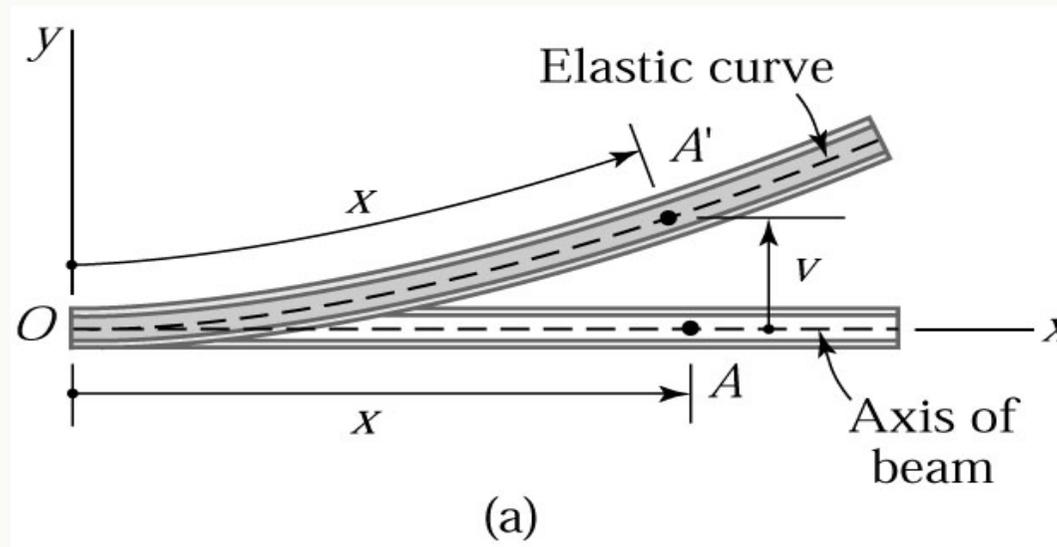
**Figure 6.1 (a) Deformation of a beam.**
