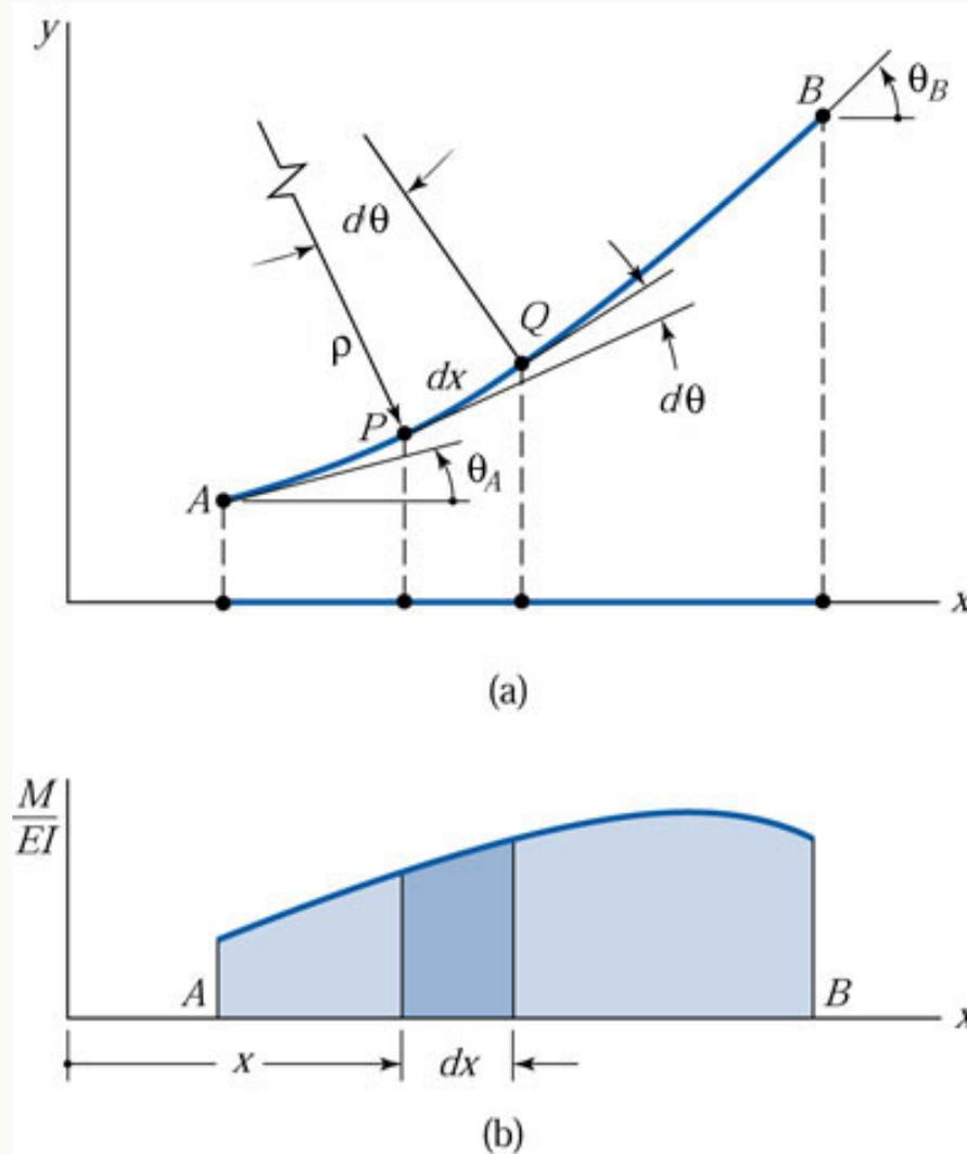
■ Because cross sections are assumed to remain perpendicular to the axis of the beam  $d\theta$  is also the difference in the slope of the elastic curve between P and Q, as shown in Fig. 6.4 (a).
