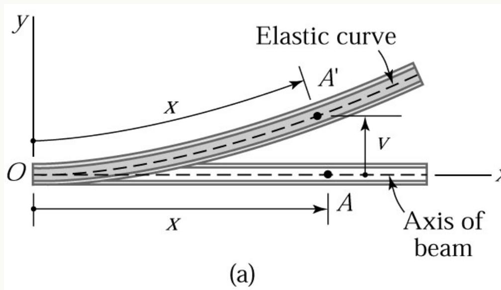
that the horizontal deflection of  $A$  is negligible provided the slope of the elastic curve remains small.
