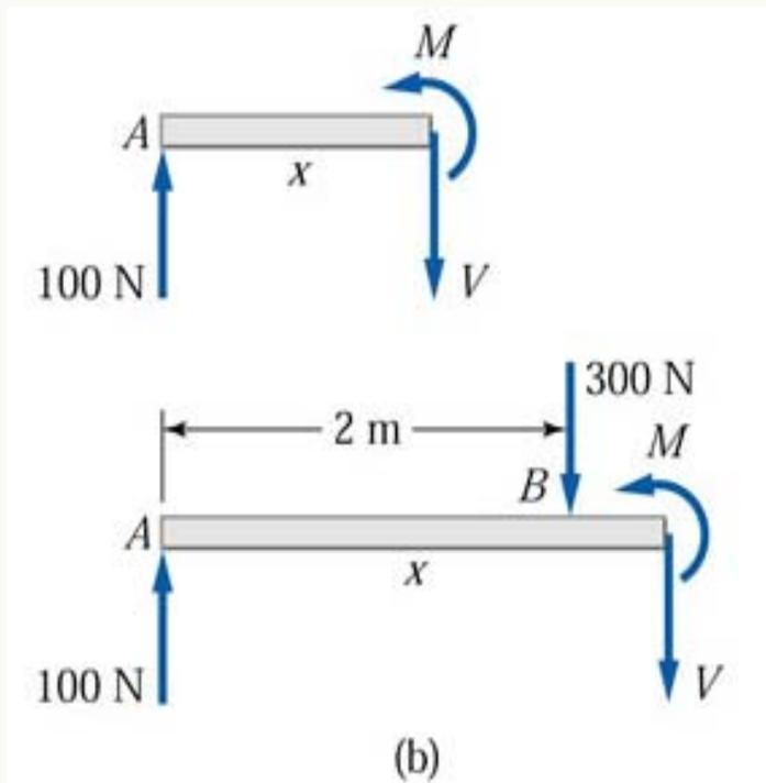
Because the loading is discontinuous at  $B$ , the beam must be divided into two segments:  $AB$  and  $BC$ . **The bending moments in the two segments** of the beam can be derived from the free-body diagrams in Fig.(b).
