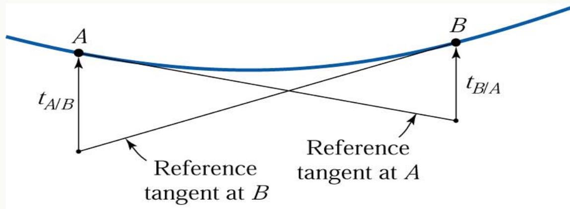
**Figure 6.6 Tangential Deviations of the elastic curve.**
