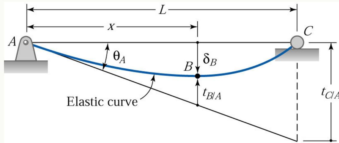
**Figure 6.11 Procedure for calculating  $\delta_B$ , the displacement of point  $B$  on the simply supported beam.**
