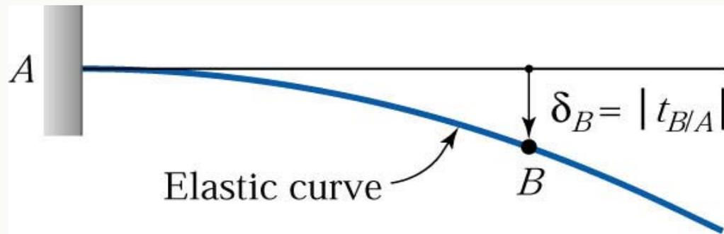
**Figure 6.10** The displacement Equals the magnitude of the tangential deviation for point  $B$  on the cantilever beam.
