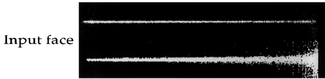
Fig. 1. Top-view photograph of a 10- \mu\text{m} soliton (upper trace) and a normally diffracting beam (lower trace) propagating along a 5.5-mm crystal.
