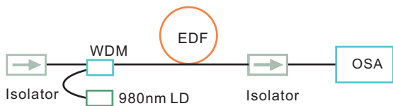
Fig.4. The configuration for the ASE measurement of the EDF.
